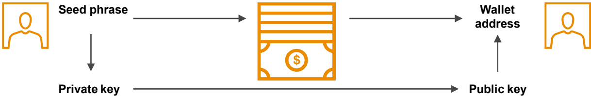
Figure 1: How a blockchain wallet works
